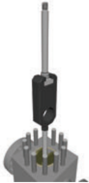
19. Remove the Gate and Stem Assembly.
