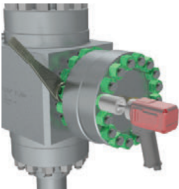
1. While holding the hex nuts on the body flange, loosen each of the test flange hex nuts.
