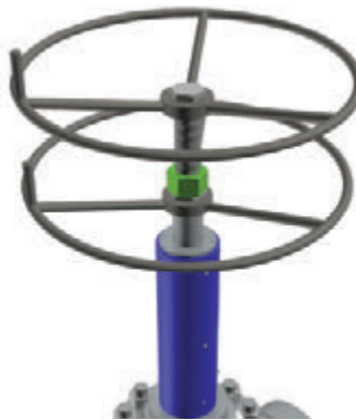
5. While holding both hand wheels tight, tighten the lock nut down to hold everything engaged.
