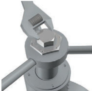
1. Remove the Backseat Gland.
