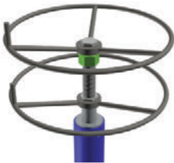
4. While one operator holds the backseat engaged, have another operator thread in the backseat tool and tighten the backseat tool hand wheel. Do not over tighten the tool.
