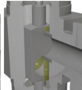
5. The gate must be fully open (left) or closed (right).
