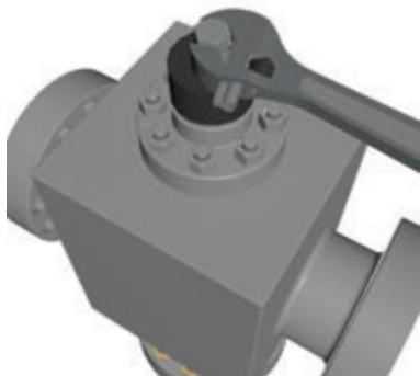
7. Using a wrench to tighten the bolt down to lock the stem/backseat into position. Do not over tighten the bolt. (Approximately 50 ft*lb)
