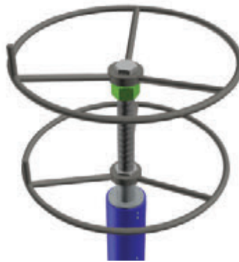
2. Carefully insert the FM Series Backseat Tool about 1 inch. Be sure the supplied nut is threaded under the hand wheel as shown.
