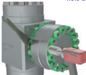
4. Torque the service flange hex nuts with a certified torque gun until they are tight.
