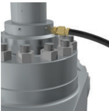
4. Remove the upper bonnet grease fitting cap, and attach a flow line from the grease pump to the grease fitting as shown above.
