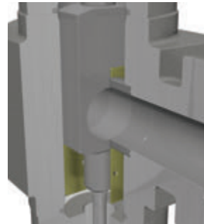
5. The gate must be fully open (left) or closed (right).
