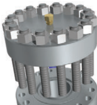
2. After removing the body flange hex nuts, you can remove the test flange, its studs, and their hex nuts.
