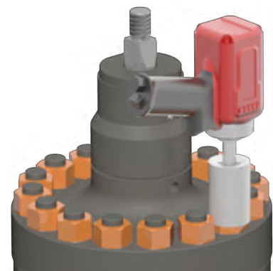
6. Unscrew and remove all Bonnet Bolts using an impact wrench.
