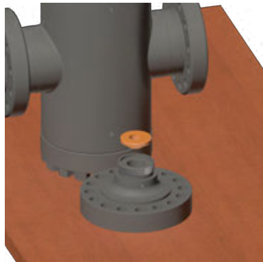
6. Remove the Packing Retainer Busing.
