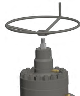
3. Remove the Handwheel.
