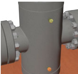
2. Be sure the lower grease fitting cap is on and tight.
