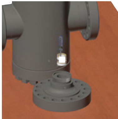
7. Remove the Stem Packing and Packing Injection Sleeve with a pick. Avoid scratching the internal wall of the Bonnet during removal.
