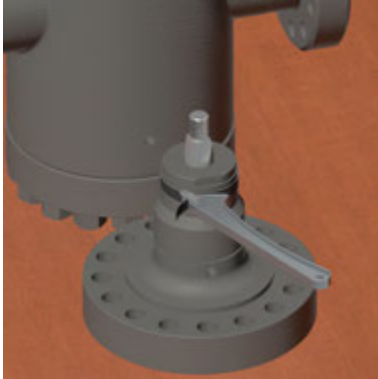
1. Unscrew and remove Bearing Housing with a strap wrench.
