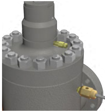
4. Screw the stem of the releasing tool into the fitting forcing the ball check off its seat. The valve will vent and drain once the ball check is unseated.
