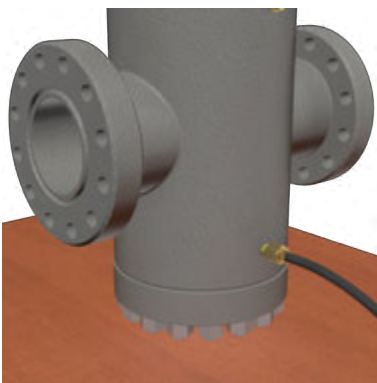
4. Remove the lower bonnet grease fitting cap, and attach a flow line from the grease pump to the grease fitting as shown above.
