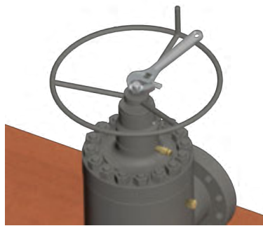
2. Unscrew and remove the Handwheel nut using a crescent wrench.
