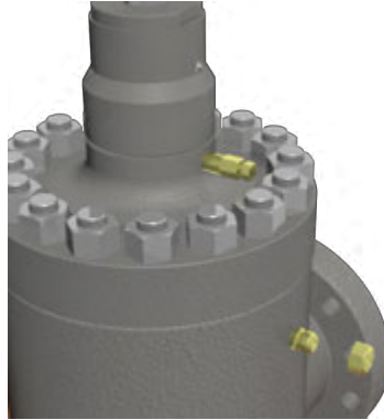
2. Remove the safety cap from either body grease fitting
