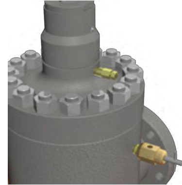
3. Attach the pressure release tool.
