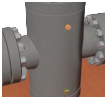
1. Be sure the upper grease fitting cap is on and tight.
