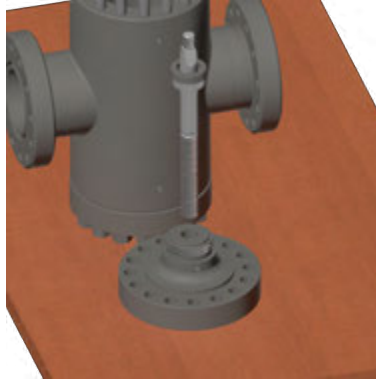
3. Remove the Stem. One of the Thrust Bearings will also be removed.
