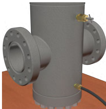
5. Remove the upper bonnet grease fitting cap, and attach a pressure release tool as shown above.
