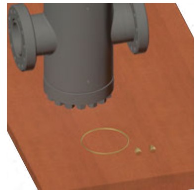
12. Remove the Bonnet Seal Ring and Grease Fittings.
