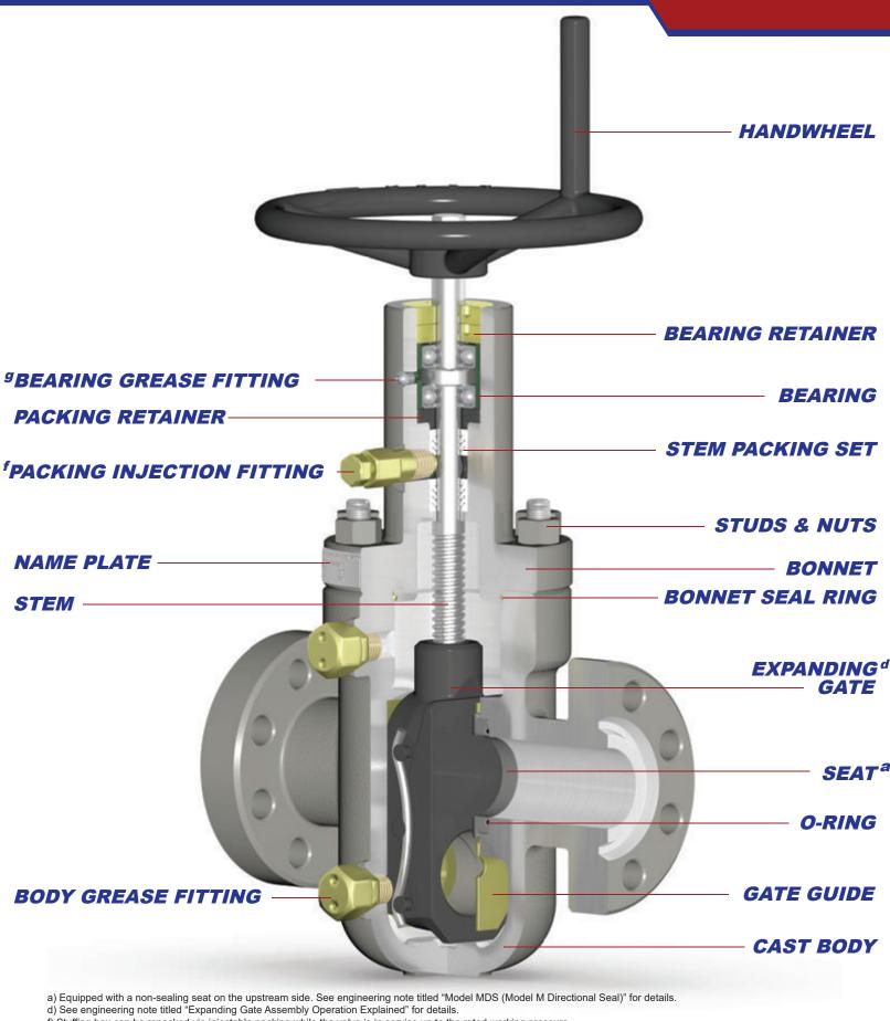
f) Stuffing box can be repacked via injectable packing while the valve is in service up to the rated working pressure.
