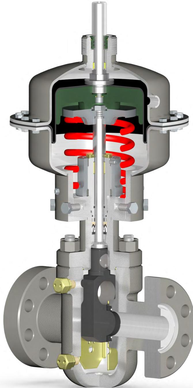
***PNEUMATIC DIAPHRAGM ACTUATOR (PDA)
